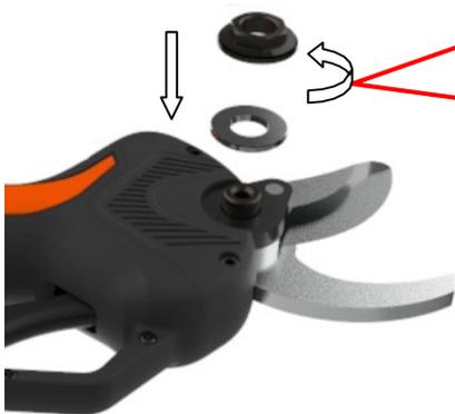
**10. Place the flat needle roller bearing as shown and screw on the locking nut.**
