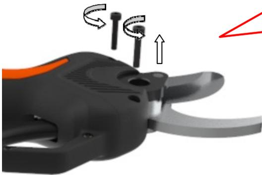
**4. Turn counterclockwise as shown in the picture, remove the M3 screw from the blade cover.**
